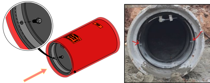
Figure 32: Style 790 Anchor Bolt/Pin Installation
